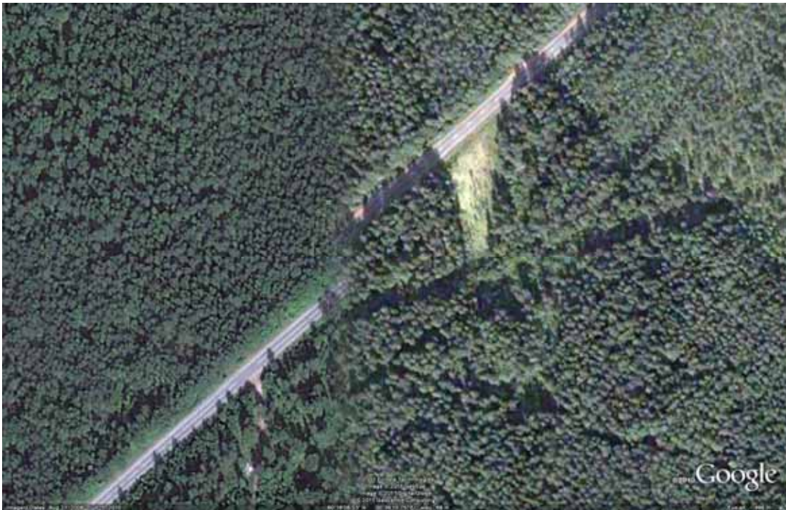
Figure 1: Geo-Registration Errors: Finding the positions in Google Earth is not without error. Notice the apparent jump in a straight road. This represents at least an uncertainty of about 10 m. This is probably from a difference in elevation angle between the two images.
