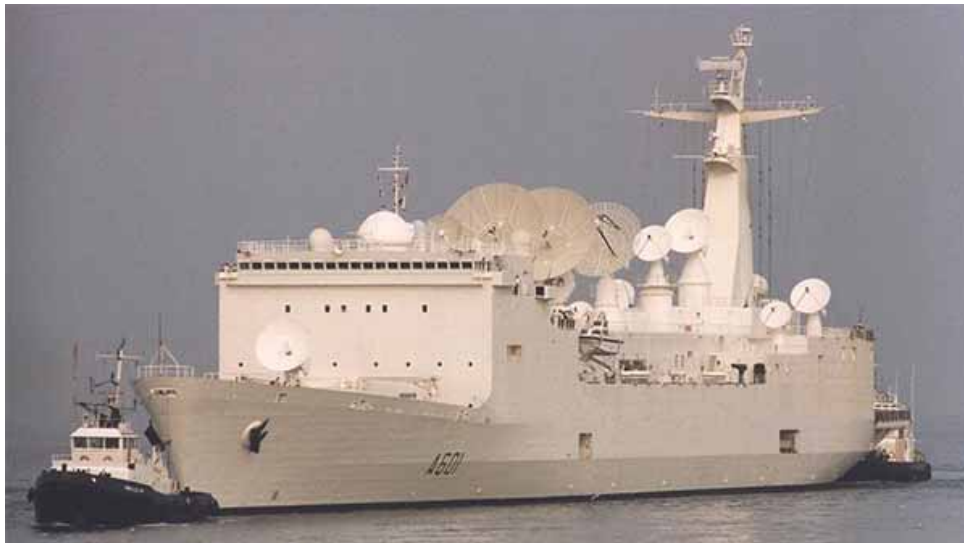
Figure 3: DGA Monge Tracking Ship: This system provides the capability to make observations from many parts of the world. (Photo from Military-today Jul 2011, http://www.military-today.com/navy/monge_ship.htm )
